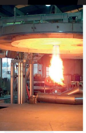
For maximum energy savings the cardanically suspended heat shield guarantees a tight sealing of the ladle.
